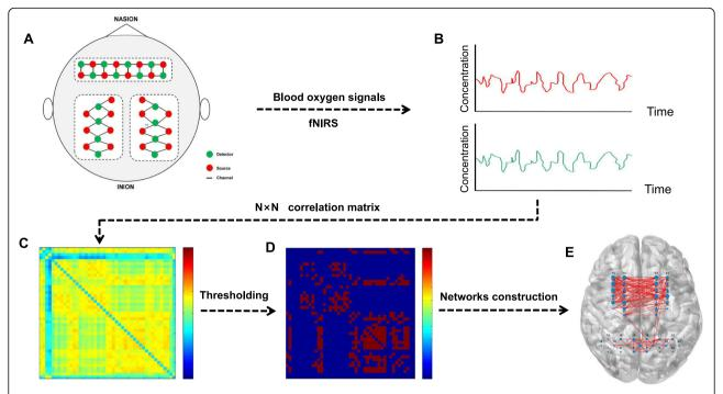
Fig. 4 The graph theoretical analysis process of fNIRS-brain networks. A Schematic illustration of the fNIRS channels layout. B fNIRS-Blood oxygen signals. C Construct a  $N \times N$  correlation matrix. D Set threshold to construct a new correlation matrix. E Brain functional connectivity
