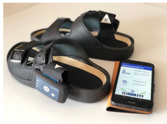
Fig. 3 Study materials for patients in the intervention group showing the sensor-equipped insole (Medixfeet Insole®, Thorsis Technologies GmbH) and the Smart Prevent Diabetic Feet Application (SPDFA)
