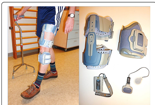
Fig. 2 The functional electrical stimulation device including two cuffs, a foot switch, and a control unit
