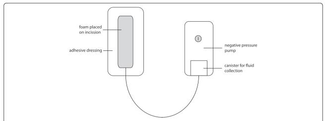
Fig. 2 Negative-pressure incision therapy wound device used in the Poniy trial. The sterile foam is placed on the skin incision immediately after skin closure and attached to the skin via the adhesive dressing. A fixed negative pressure of –75 mmHg to –125 mmHg is applied via the negative-pressure pump and the attached tubing. Wound secretions are collected in a canister, which is integrated in the pump
