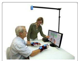
**Figure 2 Virtual reality training system setup (YouGrabber).** The model wears hand gloves with movement sensors attached. The screen displays real-time hand and finger positions.
