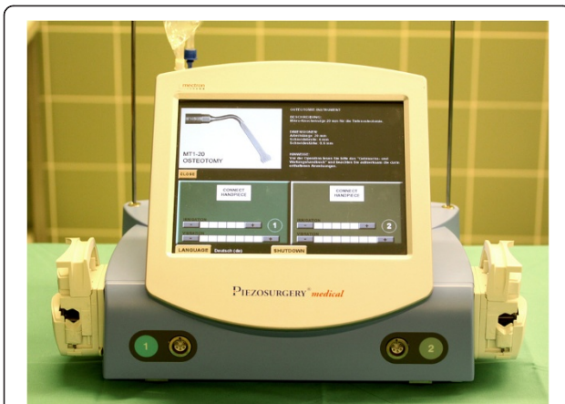
Figure 2 Piezosurgery® medical, multipurpose device uses micrometric ultrasonic piezoelectric vibrations, variable in frequency and in cutting energy. There is a therapeutic potential and benefit of the piezoelectric-assisted surgical saw in dentoalveolar surgery. Piezosurgery® enables more precise and nontraumatic cutting of bone in comparison to conventional methods (micrometric cut). The instrument vibrates with a modulated ultrasonic frequency. Because the vibration frequency of Piezosurgery® is optimal for mineralized tissue, it does not cut soft tissue. Therefore, an osteotomy with this device to remove a bony mass of the mandible prevents anatomical soft tissue injuries, such as to the dentoalveolar nerve (Figure 3).
