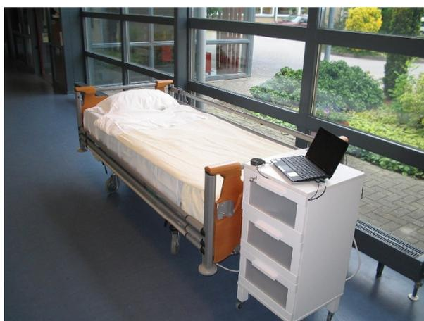
**Figure 1** High-dependency bed with PAS mattress and night table with computer which is normally locked up in the night table.
