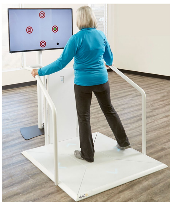
Fig. 2 Study device: Dividat Senso in action. Pressure-sensitive plate with handrails on three sides and screen on head-height of the participant, showing the video game. The participant performs a stepping movement to play the game
