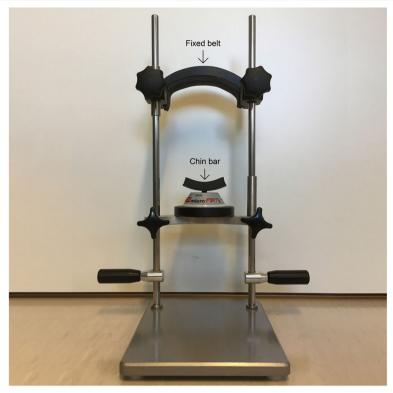
Fig. 2 Examination frame and dynamometer (MicrofetTM, Biometrics, Almere, The Netherlands)
