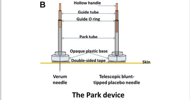
Fig. 2 Structure of the Park Sham Device. Park Sham Device with sham needle and real needle. 1. Needle handle, 2. Guide tube, 3. Guide O-Ring, 4. Park tube, 5. Flange, 6. Double sided tape, 7. Skin 8. Dermis, 9. Muscle, 10. Dull tip of sham needle, 11. Sharp tip of real needle
