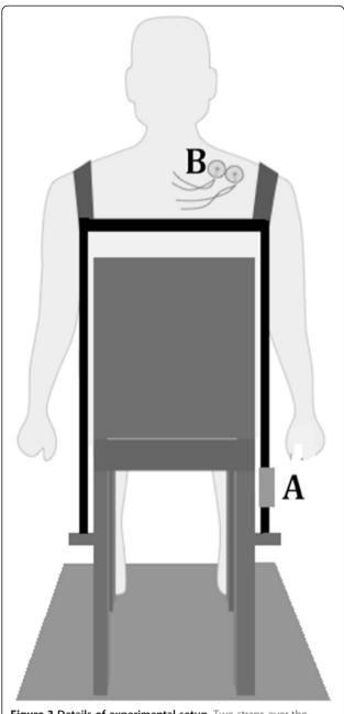
**Figure 3 Details of experimental setup.** Two straps over the acromion -one attached directly to the chair and one attached to the support of a load cell **(A)**; Force and electromyography activity **((B)** surface electrode) of the upper trapezius muscle will be measured simultaneously during shoulder elevation movements. Feedback will be provided from the projection of a 20-inch screen on a white wall in front of the subject.
